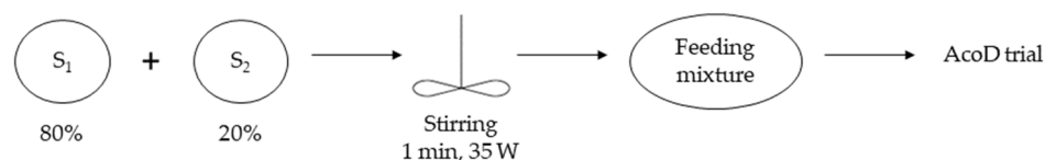
Figure 3. Feed mixture preparation for AcoD trials. Experimental conditions: mixing at 50 rpm, 35 W, for 1 min at room temperature.
