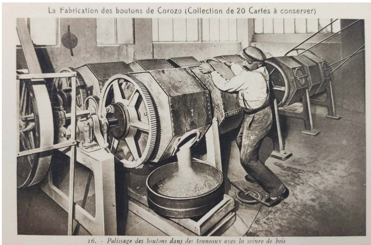
Figure 23. Polishing buttons in barrels with sawdust
