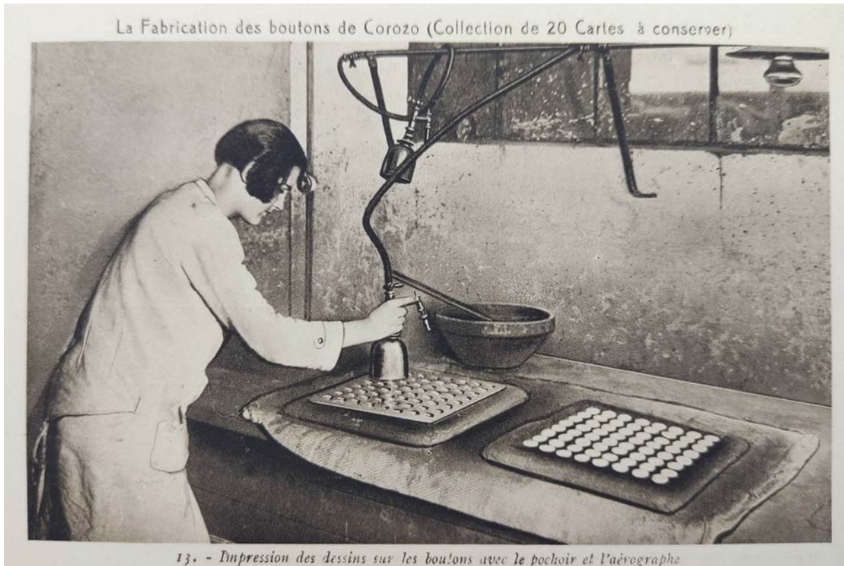
Figure 20. Printing designs on buttons with stencil and airbrush
