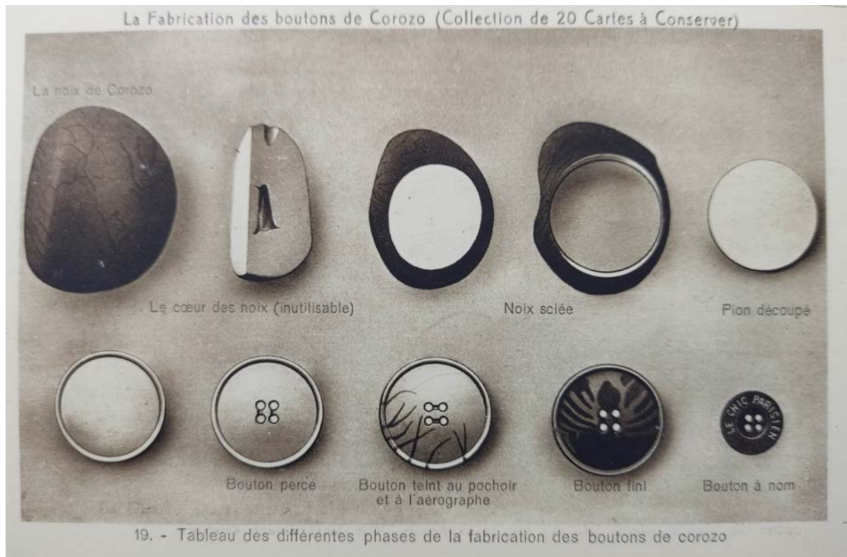
Figure 26. Table with different phases of corozo buttons' manufacture
