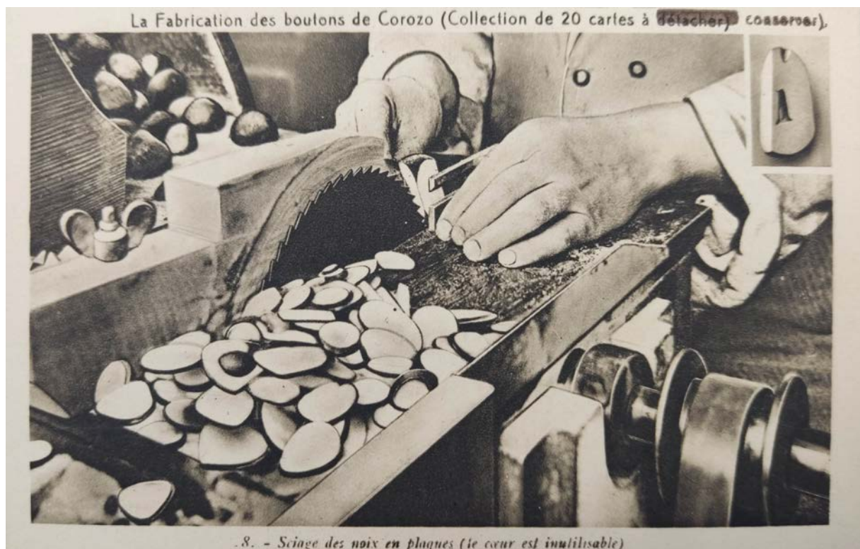
Figure 15. Sawing nuts into slabs (the core is unusable)
