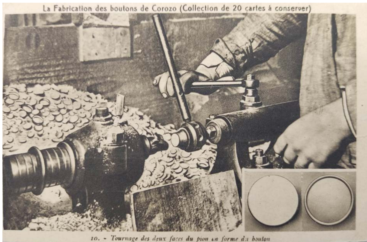
Figure 17. Turning both sides of the button-shaped pawn
