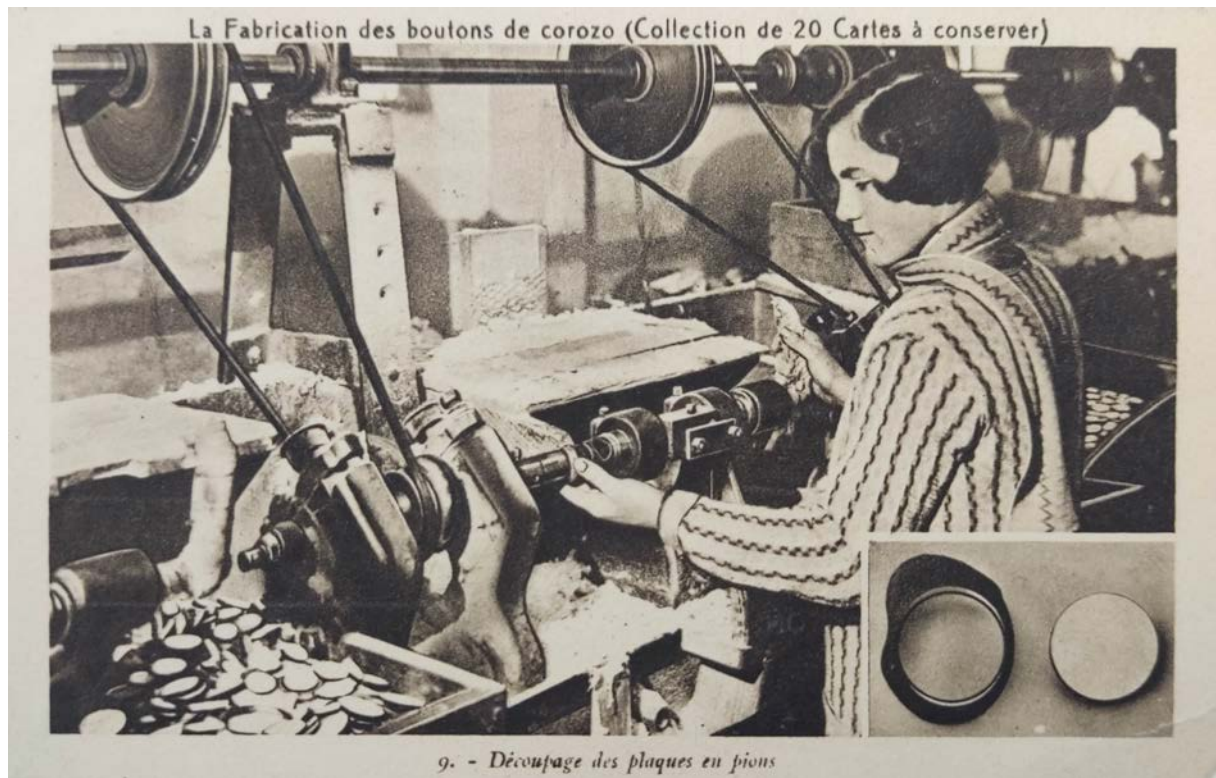
Figure 16. Cutting the plates into pawns
